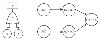
Fig. 2 An OR gate and the equivalent DEN
