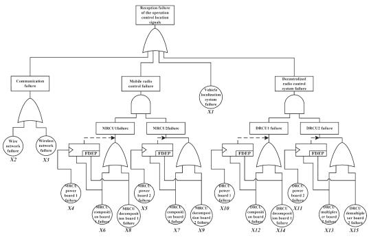
Fig. 4. DFT model of train-ground wireless communication system
