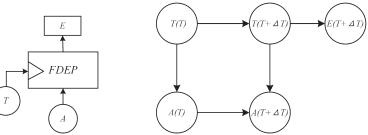
Fig. 3 An FDEP gate and the equivalent DEN.
